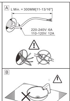
It is recommended to avoid installation of dryer near high reflective objects (mirror, stainless steel washbasins, etc.) in order to avoid faulty function of the presence sensor.
