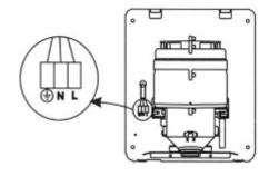
Drill four 7mm holes in the wall to a depth of 40mm. Insert the raw plugs into the holes and secure the unit on the wall with the screws.
