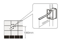
Remove the cover by using the allen key provided to undo the two screws.
